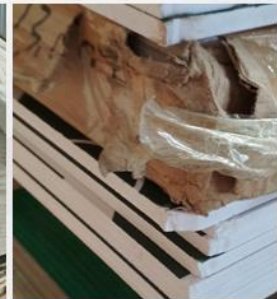
PVC foam board tends to brake during handling or during delivery if not well protected.
